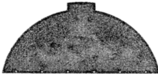
Fig. 3. Element mesh of the 2D model of the greenhouse.
